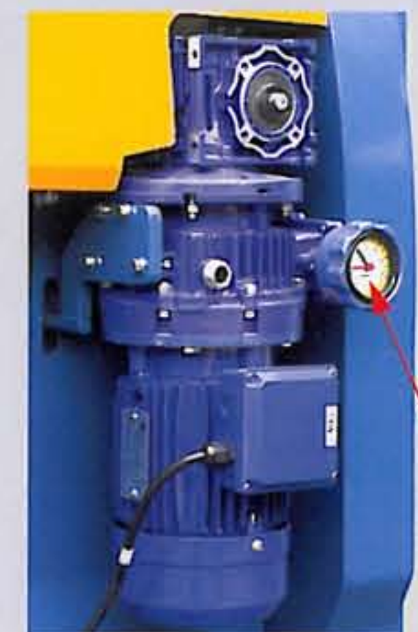
Feed Speed Change Knob With Indicator
